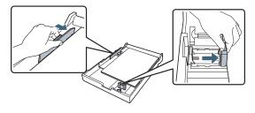
Insert the paper cassette. Push it firmly into the printer.
